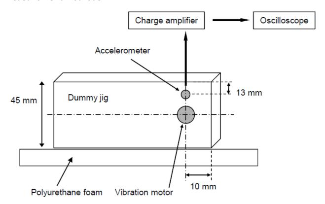
Specification of the dummy Jig
